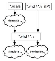
As SpinalHDL is interoperable with VHDL and (System)Verilog, you can both instantiate SpinalHDL IPs in these language (using generated code) and instantiate IPs in these languages in SpinalHDL (using BlackBox).
