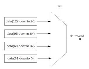
Example for muxListDc selecting bits from a configurable width vector:
