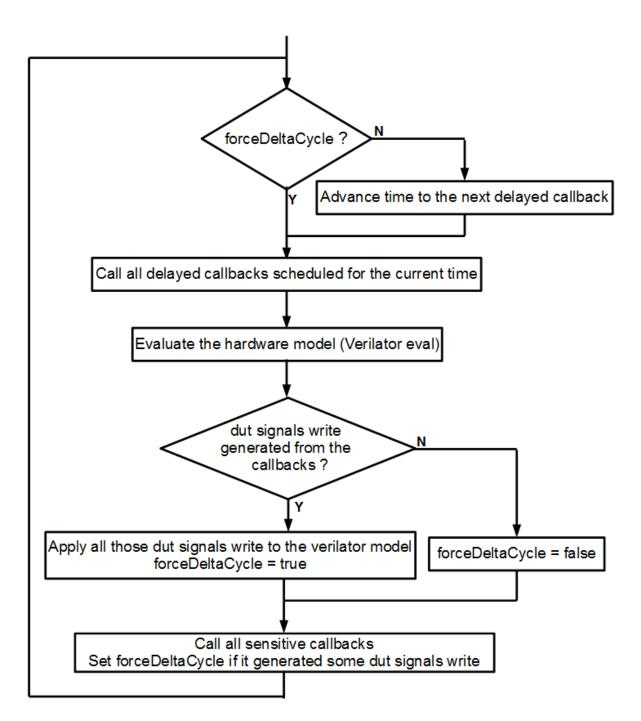
At a low level, the simulation engine manages the following primitives:
